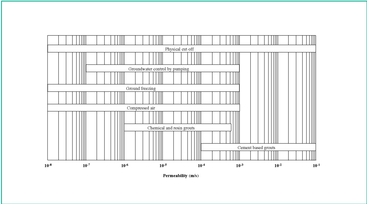
FIGURE B.1: APPROXIMATE RANGE OF APPLICATION OF GROUNDWATER CONTROL TECHNIQUES IN SOILS
